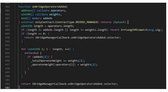
Figure 6 onBridgeOperatorsAdded function screenshot
